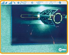
During a simulated weld sequence, visual graphical aids guide user to achieve adherence to parameters.
